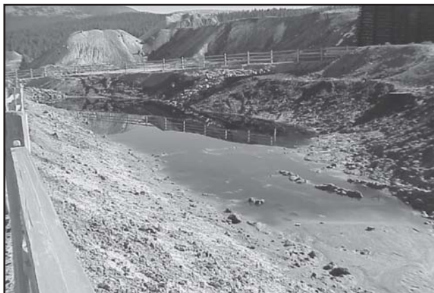
FIGURE 6.2 Acid drainage–affected waters and waste rock, Leadville, Colorado
