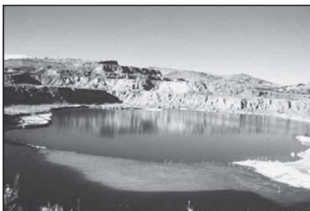
FIGURE 6.3 Pit lake at the Copper Flat mine, Hillsboro district, Sierra County, New Mexico. Many porphyry copper deposits are mined by open pit methods and result in pit lakes that have low pH values. The pH of this lake varies seasonally from 4 to 6.
