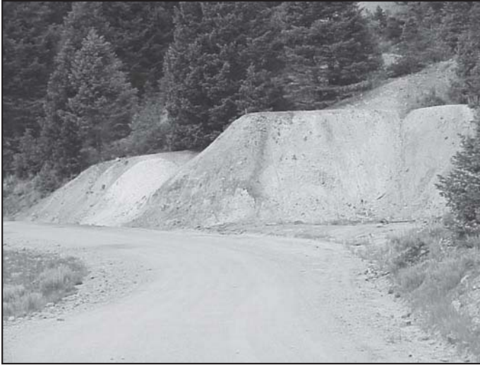
FIGURE 5.4 Oxidized waste piles can be sources of MIW (Comet mine site, Boulder River, Montana)
